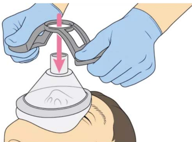
Figure. The Mask Ventilation Grip is placed over any standard valve mask.
